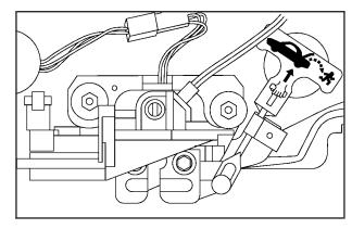
There is a glow-in-the-dark emergency trunk release handle located inside the trunk on the latch. This handle will glow following exposure to light. Pull the release handle up to open the trunk from the inside.
